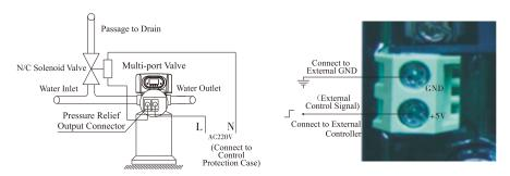
Figure 3-10 Wiring of Pressure Relief Output
