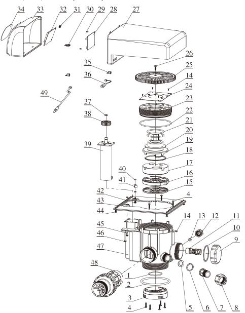
Component and part No. for F74A3/F74A1 (Components for F74A1without No.48 and No.49)
