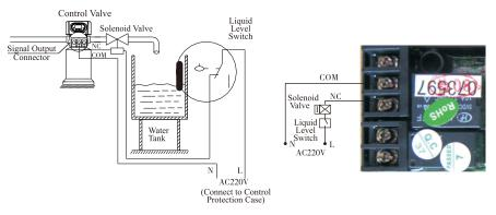
Figure 3-1 Wiring of Solenoid Valve on Outlet
