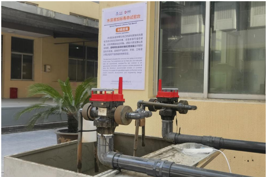
Water-Fertilizer Solution Resistance Test (Double concentration)
