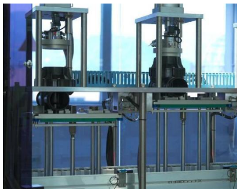
100% air tightness test
