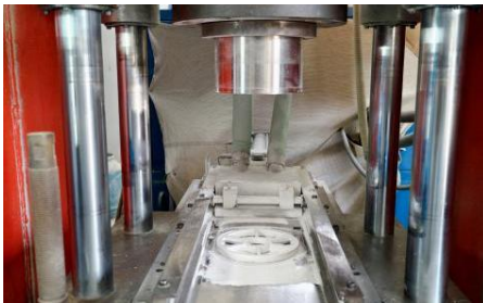
Ceramic Disk Dry Pressing
